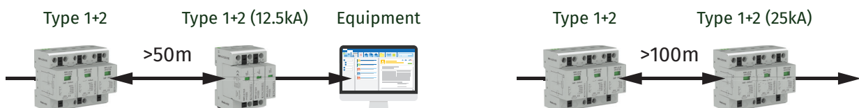
Figure SPD:10. Type 1+2 devices protective distances
